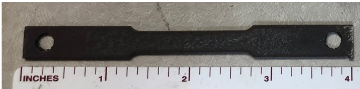
Figure 2.1 ASTM E8 sub size dog bone sample for Gleeble heat-treatment and Instron tension testing [49].
